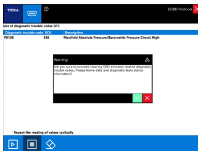
Figure 126: Error Clearing Mode $04
