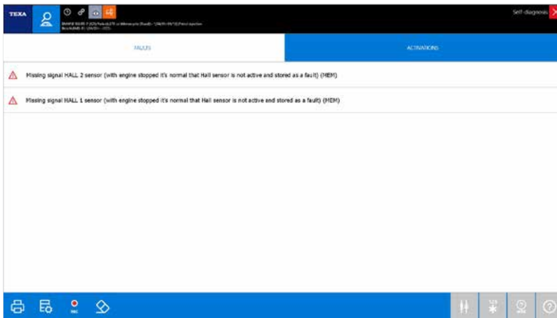
Figure 43: The error page always indicates the missing signal to the HALL sensors
