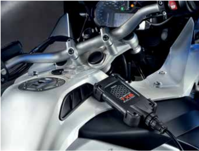
Figure 9: NAVIGATOR TXB Evolution allows the recording of the diagnostic session in "Dynamic Testing" mode
