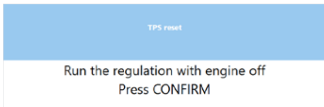
Figure 165: Start the process with the engine OFF
