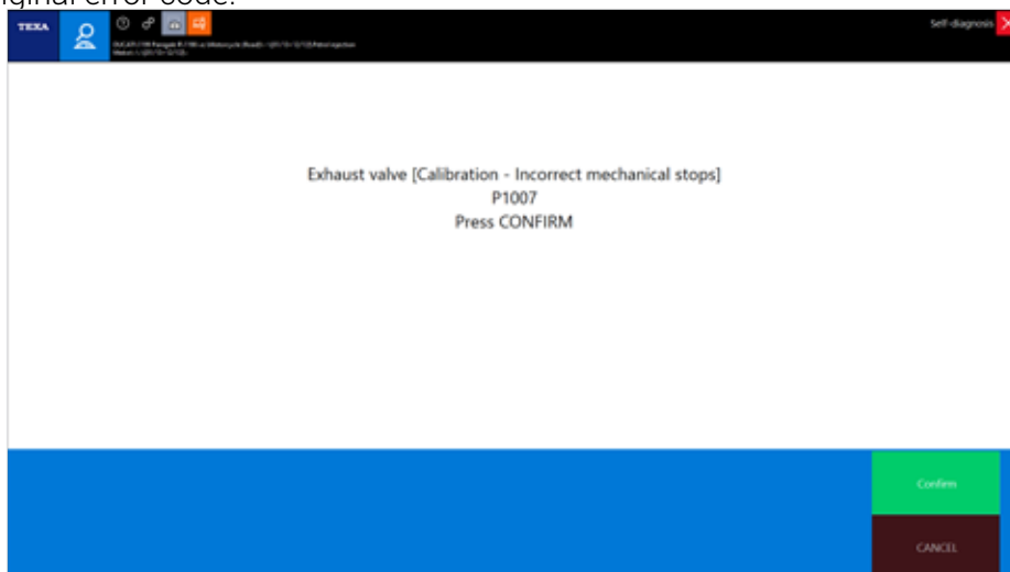
Figure 59: The DTC detail is always available by double clicking. In this case the error code P1007 indicates that the exhaust valve has a mechanical problem in the rest position
