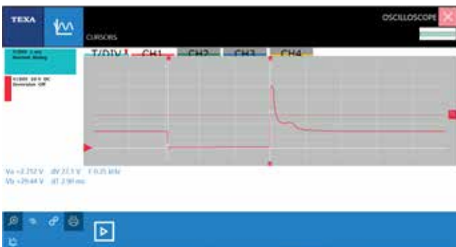
Figure 6: Oscilloscope acquisition of the opening signal of an injector
