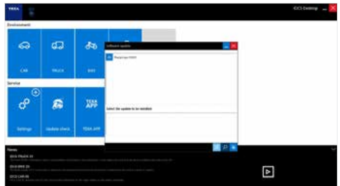
Figure 90: When the IDC5 software is started, if updates are available, a window is displayed with the possibility to download the mappings
