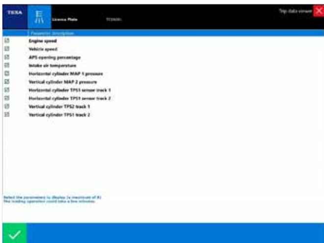
Figure 78: It is also possible to select which parameters to view from the recording group created
