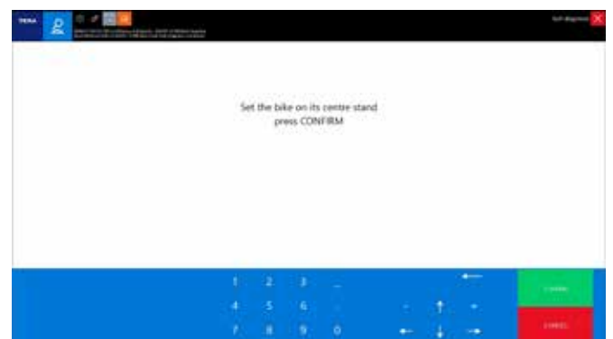
Figure 40: The IDC5 software before the actual diagnostic phase may require special conditions: in this case you will be required to place the bike on its center stand
