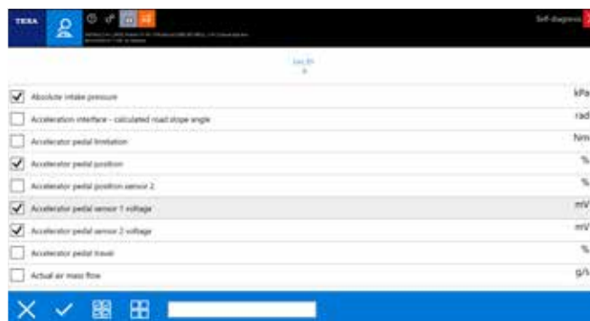
Figure 68: From the complete list of parameters you can select only those needed to create the logical group
