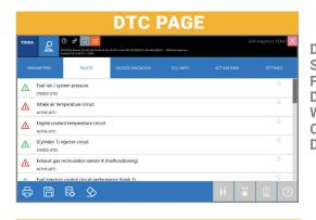
Detailed Vehicle System Listed Faults Instantly Display All Errors With Related Codes / Detailed Descriptions
