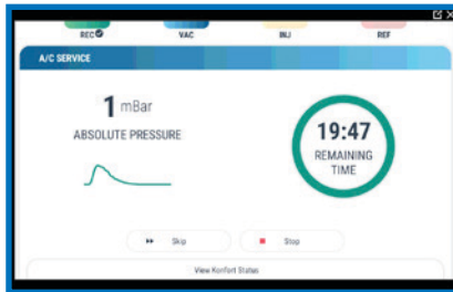
VACUUM - Leak Check / Status
